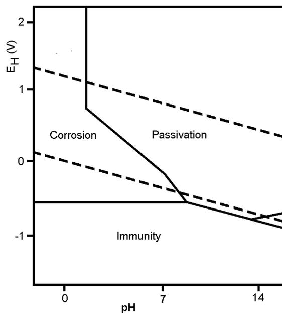
Figure 7: Theoretical conditions of corrosion, immunity and passivation by the formation of oxides. This diagram is valid only in the absence of substances with which iron can form soluble complexes and insoluble compounds
