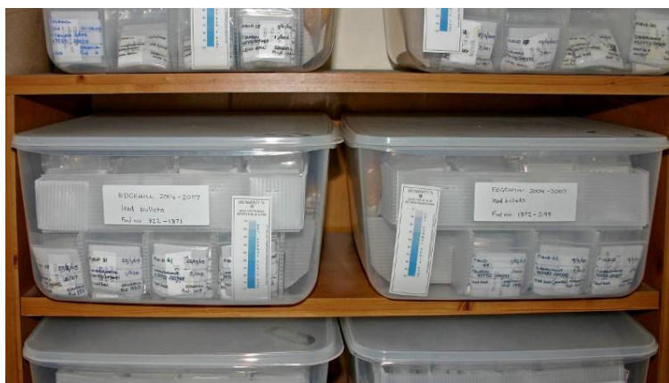
Figure 4: Storage in Stewart Boxes with indicator strip to monitor humidity. On left adequate humidity level shown by fully blue strip. The box on the right was recently opened and so temporarily has increased humidity, indicated by pink colour at top of indicator strip
