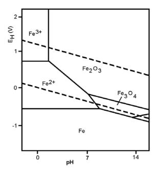
Figure 6: Simplified Pourbaix diagram (Potential –pH) for iron-water at  $25^{\circ}$ C. Fe, Fe<sub>2</sub>O<sub>3</sub> and Fe<sub>3</sub>O<sub>4</sub> are solids, while Fe<sup>2+</sup> and Fe<sup>3+</sup> are in solution<sup>22</sup>
