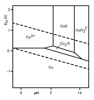
Figure 8: Simplified Pourbaix diagram (Potential -pH) for copper-water at 25<sup>o</sup>C. (to left) Cu, Cu<sub>2</sub>O and CuO are in solid phase, while Cu<sup>2+</sup> and CuO<sup>2-</sup> are in solution
